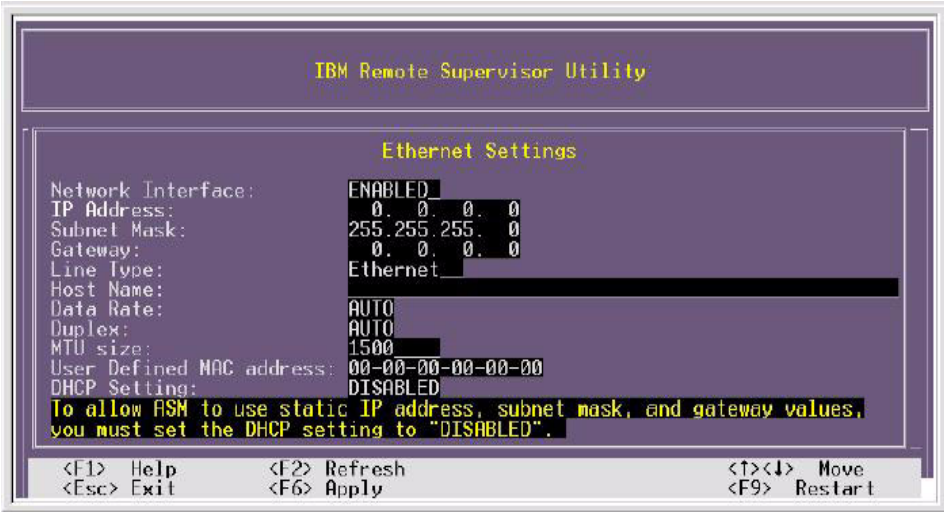
Figure 5-6 IBM Remote Supervisor Utility - Ethernet settings
